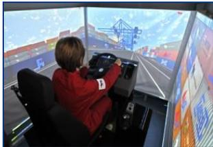
**ST-VP** is fully containerized real-time distributed HLA Simulator reproducing Port Operations. ST-VP is integrated in a 40' High Cube Container ready to be used on site immediately after arrival.
