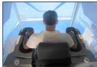
**ST-VP** Simulator allows to operate all the different Port Cranes in a Virtual World by an immersive Cave (270° Horizontal and 150° Vertical), reproducing Sounds, Vibrations, Motion in all weather conditions
